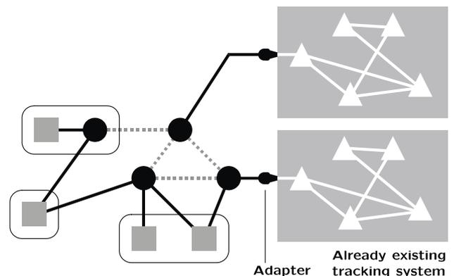
Figure 5 – Coupling of already existing components and networks to TraSer nodes
