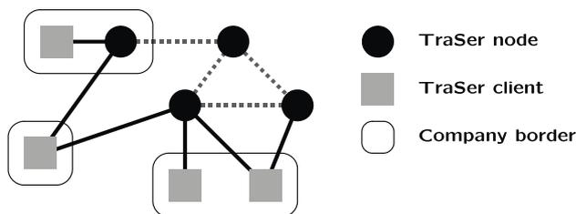
Figure 4 – Composition of a TraSer network consisting of nodes and clients
