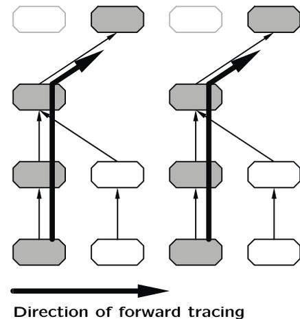
Figure 1 – Forward tracing in a gozinto graph of individual items
